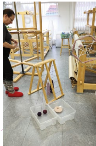
Wind 4 single or double yarns at the same time (5 - 6 single yarns) = 1 portee.
