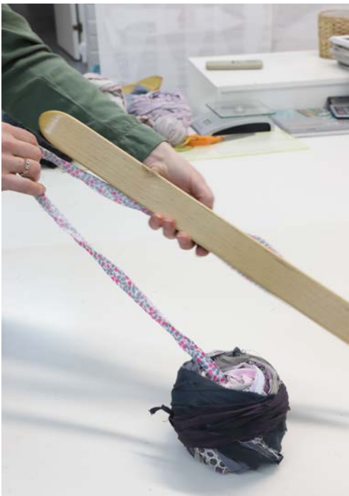
Weave a stripe from dark to light: Wind the weft on the shuttle from the light end from centre of the ball. The dark end turns last on the shuttle and colour repeat is from dark to light while weaving.
