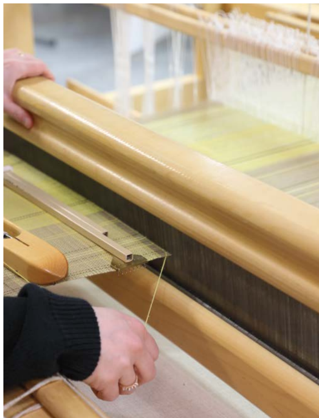
Draw thread slowly into place with the beater. The weave has same number of weft picks to warp threads per cm.
