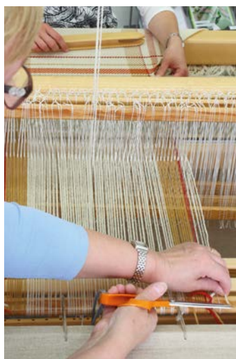
1. The helper cuts the warp thread.
