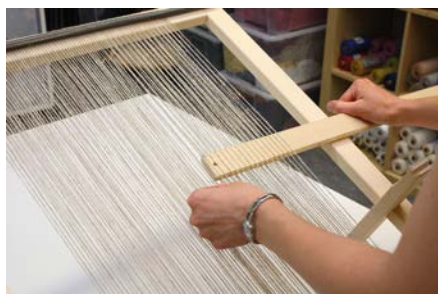
Pick every other thread onto the stick.
