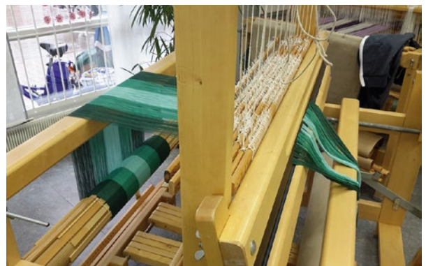
The new warp has been wound onto the beam and is ready for tying the warp on apron rod.
