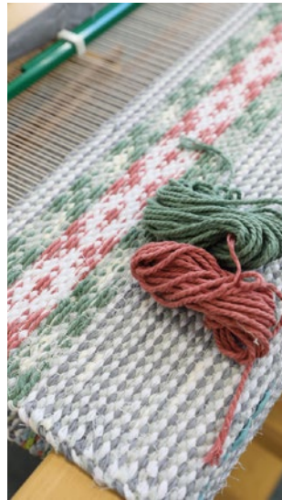
The pattern weft is a thick tightly twisted cotton mop yarn, Moppari.
